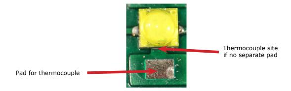
It is not required to use a solder footprint for the thermal pad that is larger than the XLamp XB-D LED itself. In testing, Cree has found such a solder pad to have insignificant impact on the resulting  $T_s$  measurement.
